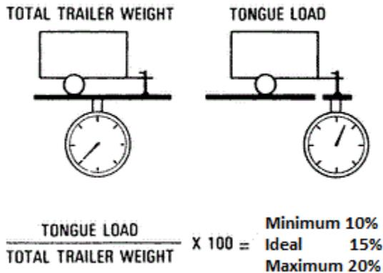
The drawing to the left illustrates the proper weight distribution for loading a trailer. Use the Weigh Station scale to achieve a minimum of 10% to a maximum of 20% of the total trailer weight of the trailer as tongue weight. A proportional tongue weight provides the best handling for addressing trailer sway. Reasonable driving speeds and proper tire inflation are equally important.
